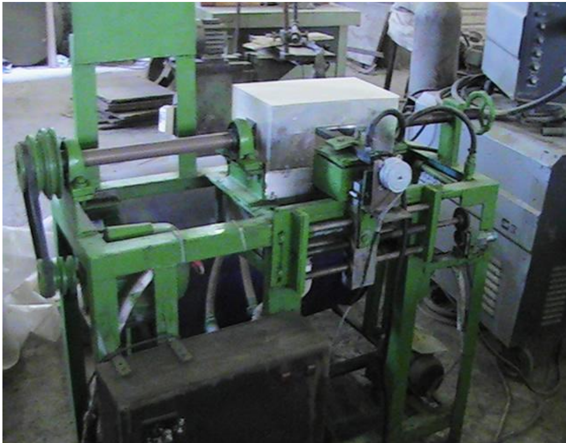
Fig. 3.5 The body of electrochemical turning machine
